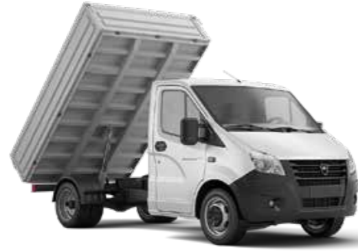
Dump truck with three-way unloading
